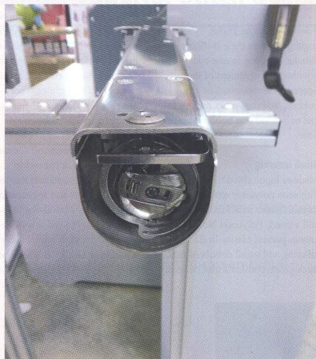
● The tubular arm of the Sprint 6 works without a picker at the front.
